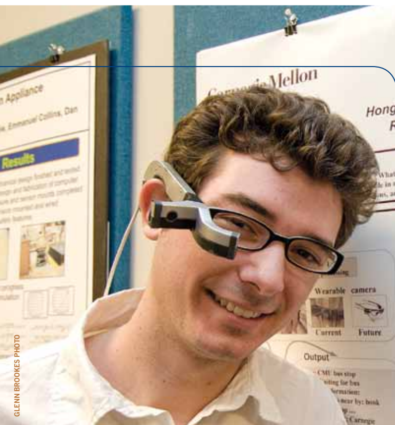
"First-Person" or "Inside-Out" vision devices that can see exactly what a person is looking at can help a robotic assistant to predict what tasks that person is trying to perform. Wearing a prototype eyepiece is Michael S. Devyver, a member of the research staff at the Robotics Institute.
