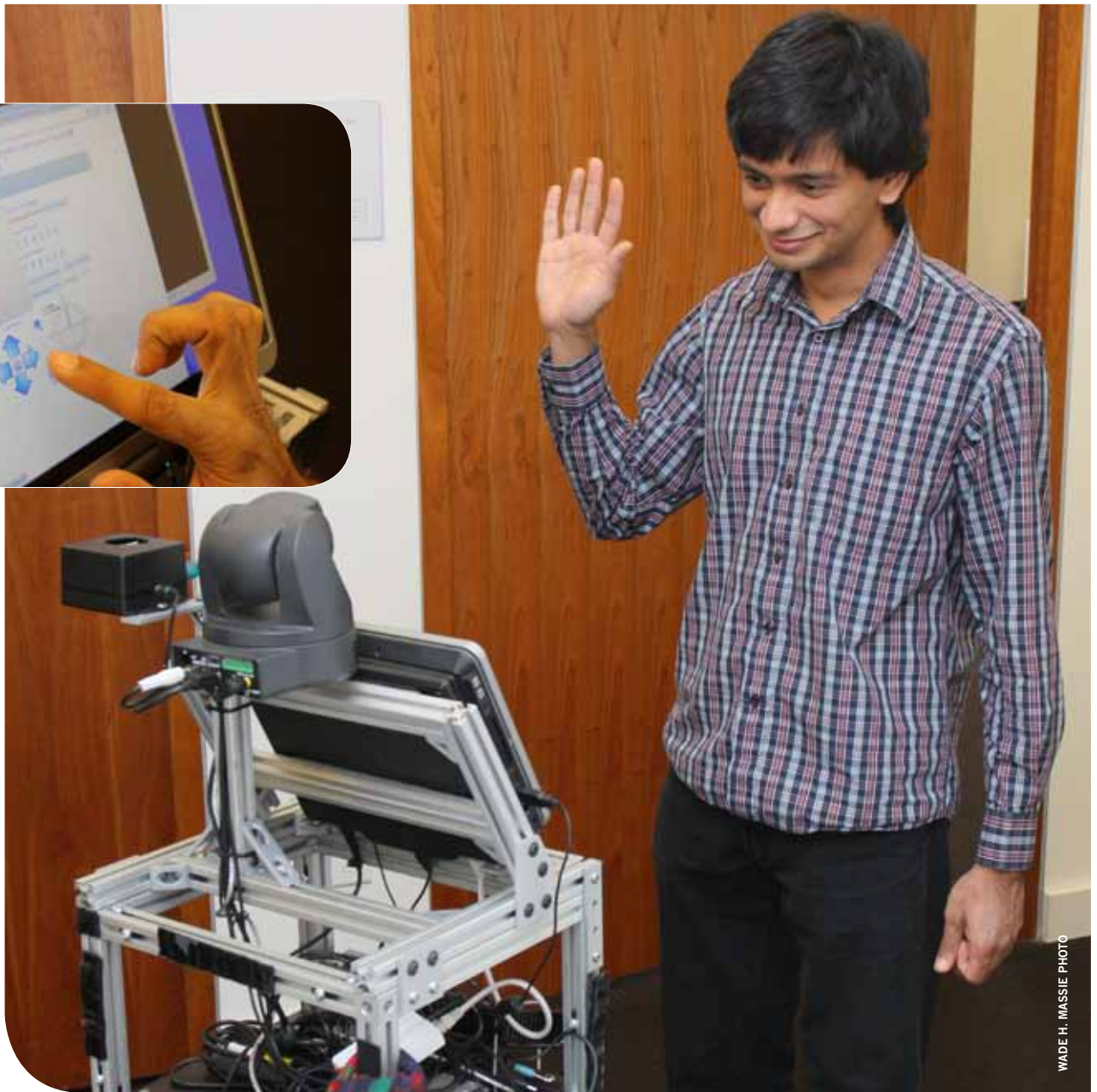
Robotics master's student Joydeep Biswas demonstrates the user interface of CoBot 2, one of the social robots under development in Manuela Veloso's CORAL lab. CoBot 2's telepresence capability will allow it to serve as a virtual stand-in for a human located anywhere in the world.
